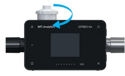
2. Screw the oxygen sensor clockwise into the appropriate port. Make sure the sensor seals off the port and there is no leak.
