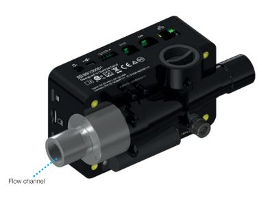
Figure 2: Flow channel
