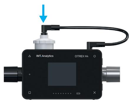
Figure 8: Oxygen sensor cable
