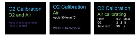
Figure 25: Screen displays "Calibration Air"
