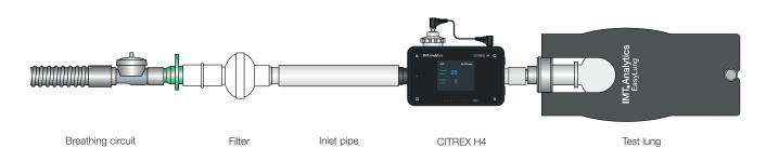
Figure 29: Measurement setup for checking ventilators
